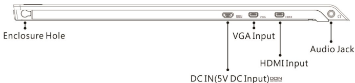
Fig.: On-Lap 2501 Series input/output ports
