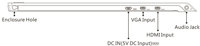
Fig.: On-Lap 2501 Series input/output ports
